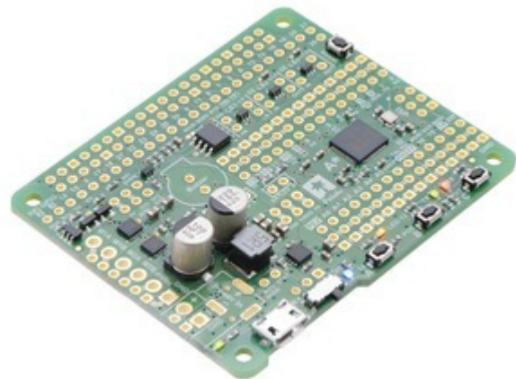
A-Star 32U4 Robot Controller SV with Raspberry Pi Bridge (SMT components only).
